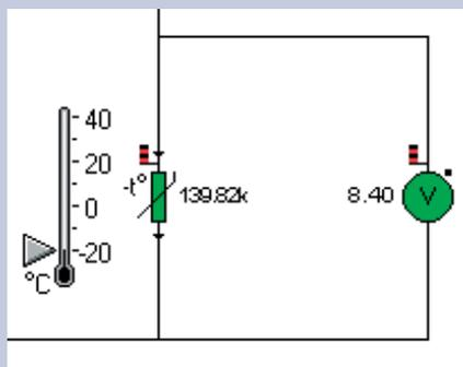
In this example, using Crocodile Technology, the thermistor has a resistance of 8.22k at 40°C producing a signal output of 4.06V, at -20°C the output signal is 8.40V. Between 40°C and -20°C the thermistor produces a varying voltage signal.
