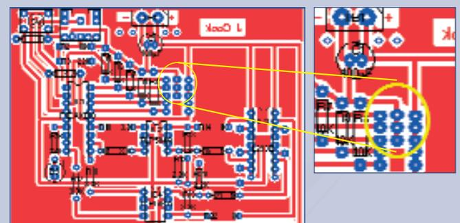
The three holes allows two resistors (that form a potential divider) to be connected between the positive and zero voltage rails. The inputs can also be used as digital inputs by ignoring the centre zero voltage holes in the middle. There are three analogue inputs on PICAXE 18 as shown previous and just one input for PICAXE 08.
