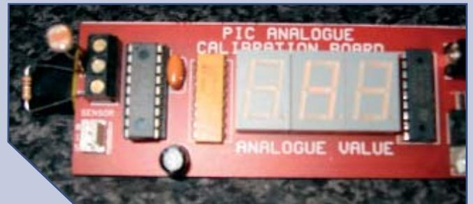
The most common input arrangement for LDRs and thermistors, is a potential divider arrangement. Potential dividers are made from resistors connected in series between the +V and 0V supply lines of a circuit.
