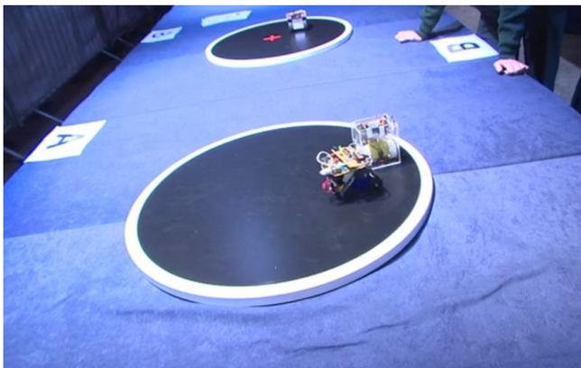
The table is big enough to ensure that operators are far enough back from the robots so as not to affect IR sensors.
