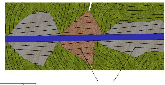
In a sloping road the lines on the cut/fill surface will always be at an angle to the edge of the road
