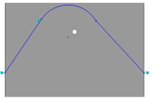
Select the line segment and arc by holding down the 'CTRL' key and apply a 'Tangent' relation
