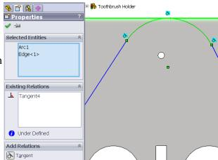
Apply a 'Horizontal' relation between the endpoints of the line segments and the points of tangency in turn.
