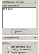
Move the cursor to the origin and select. The part origin will snap to the assembly origin.
